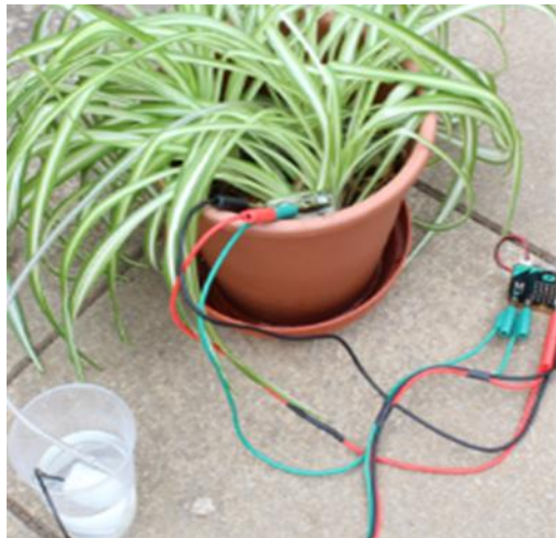
Project 2: Auto plant watering system
