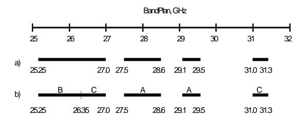
Figure 1: Spectrum proposed by IDA for broadband fixed wireless access (a) and a suggested band segmentation plan (a) for three licenses (A, B, and C).
