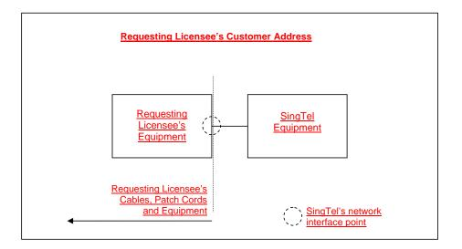
SingTel Comments: Diagram illustrates how the Requesting Licensee's associated cables and patch cords to SingTel's network interface points will connect and interface with the corresponding cabling and connectors between the Requesting Licensee's equipment and SingTel's network interface points.
