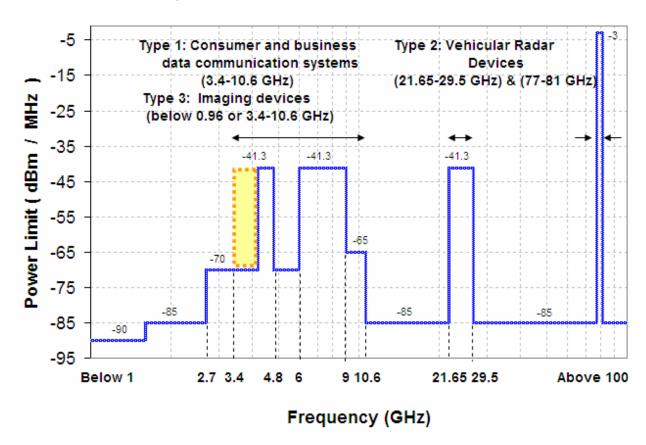
Note: UWB devices with mitigation techniques are allowed to operate at a level of -41.3 dBm/MHz in the frequency band from 3.4 to 4.2 GHz. Otherwise, the emission limit is capped at -70 dBm/MHz.
