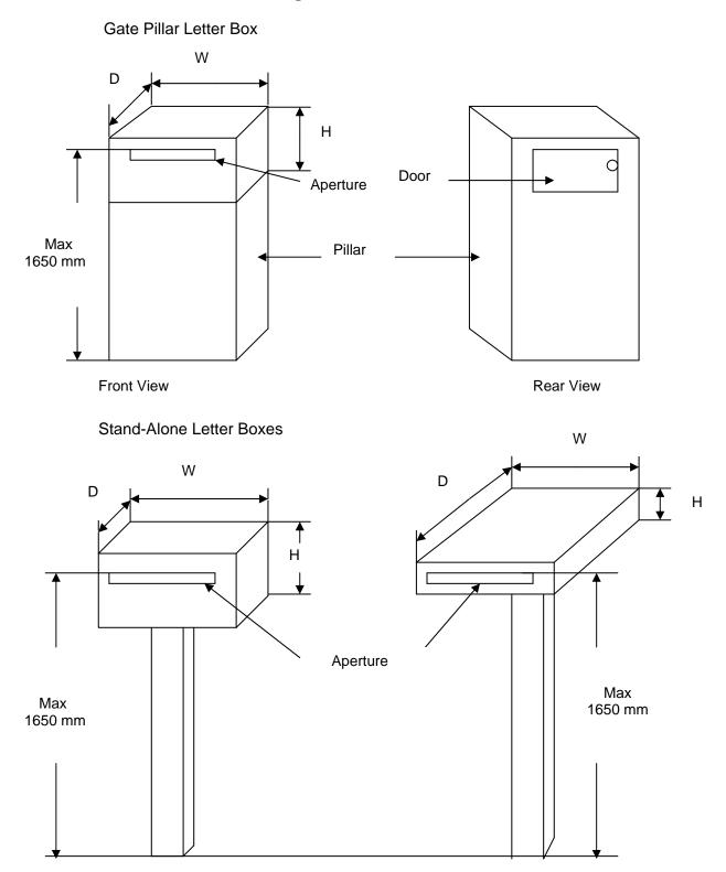
NOTE : All dimensions are internal dimensions (mm)
