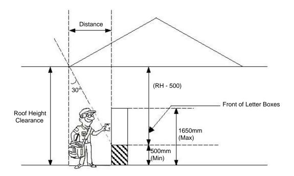
**WEATHER SHELTER** Distance =  $\tan 30^{\circ} x$  (RH-500), and Min. Distance = 1200mm
