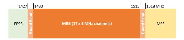
While benefitting compatibility with the MSS, this plan, compared to other options which place only 1 MHz guard band at the upper edge of the IMT band, would require less significant power constraints and/or more easily achievable filter requirements on the lowermost and uppermost IMT channels.
