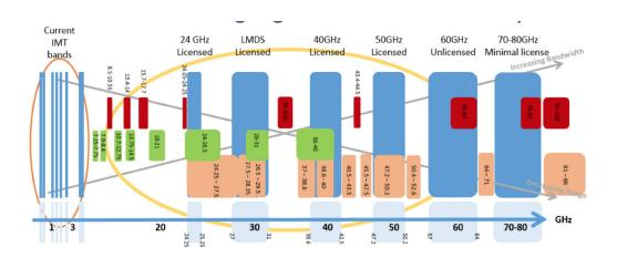
60GHz mmWave is used in WiFi 802.11ad/ay specification and standard. It uses beamforming technique for wireless communication. With the abundant of bandwidth in this frequency band, fast wireless transmission of > 10Gbps is attainable.
