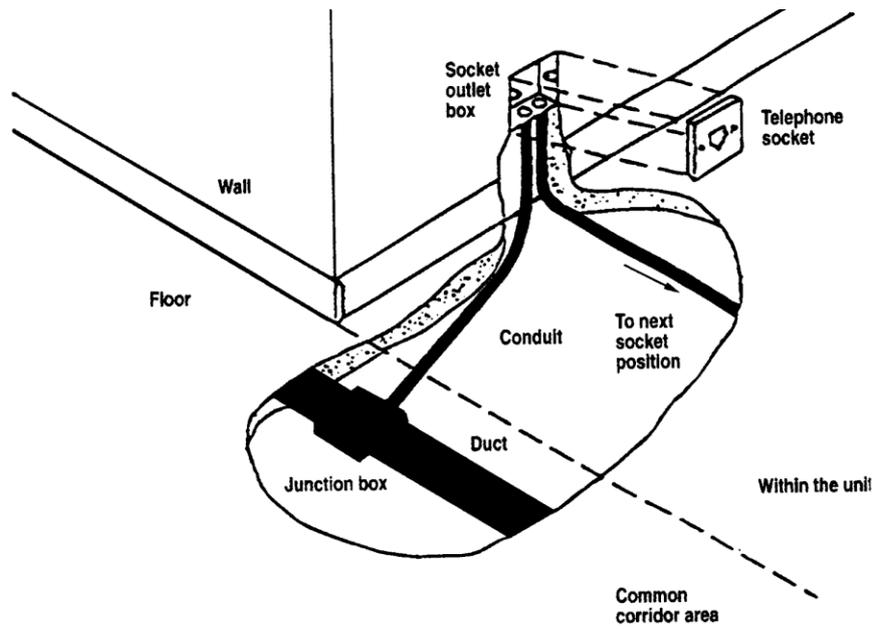
**Figure 7.29: Using conduits to distribution cables**
