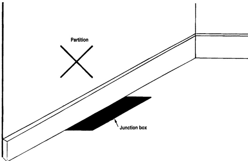
**Figure 7.11: Access to junction box for carpeted floor**
