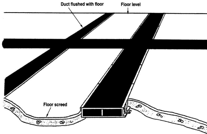
**Figure 7.4: Under-floor duct extended to floor trench / flush trunking**
