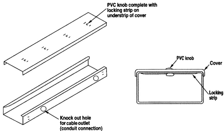
**Figure 7.28: Combination of duct & conduit distribution system**
