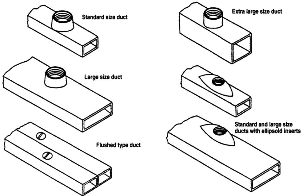
**Figure 7.8: Junction boxes installed 6m apart**
