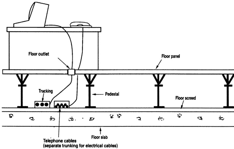
**Figure 7.15: Sectional view of a cellular floor system**
