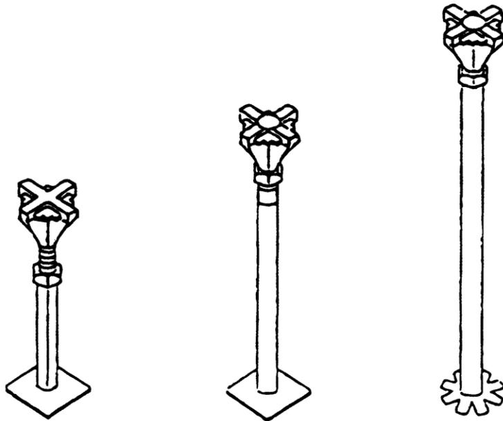
**Figure 7.14: Typical section of raised floor system**
