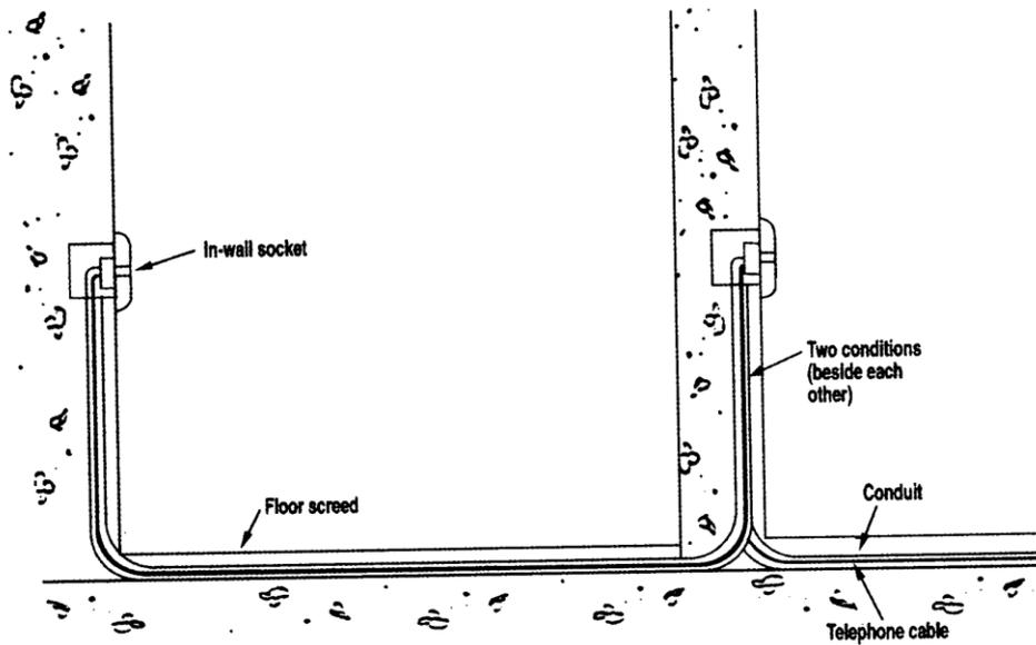
Figure 7.30: Floor duct extended into telecommunication riser
