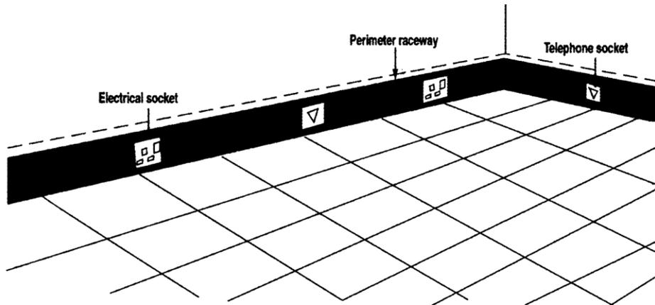
**Figure 7.22: Section of a 3-compartment skirting trunking**
