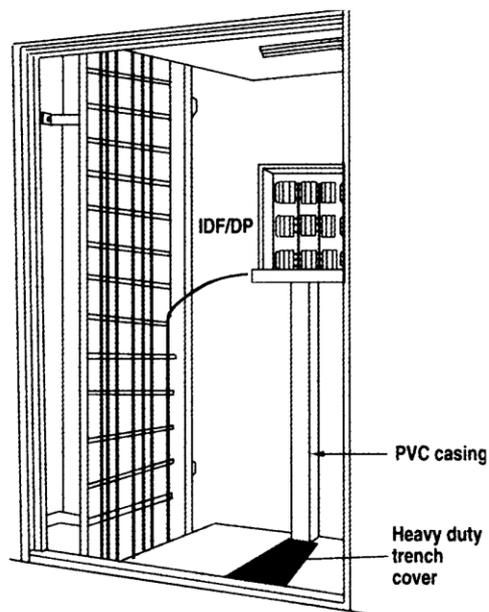
Figure 7.5: Floor trench in centre of riser
