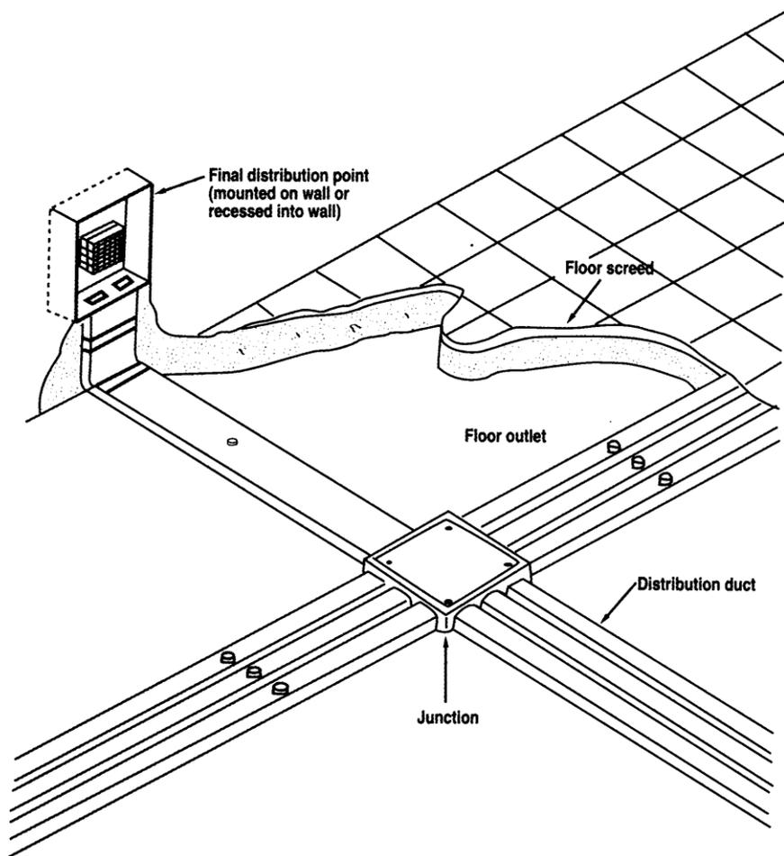
**Figure 7.3: Trench duct system**
