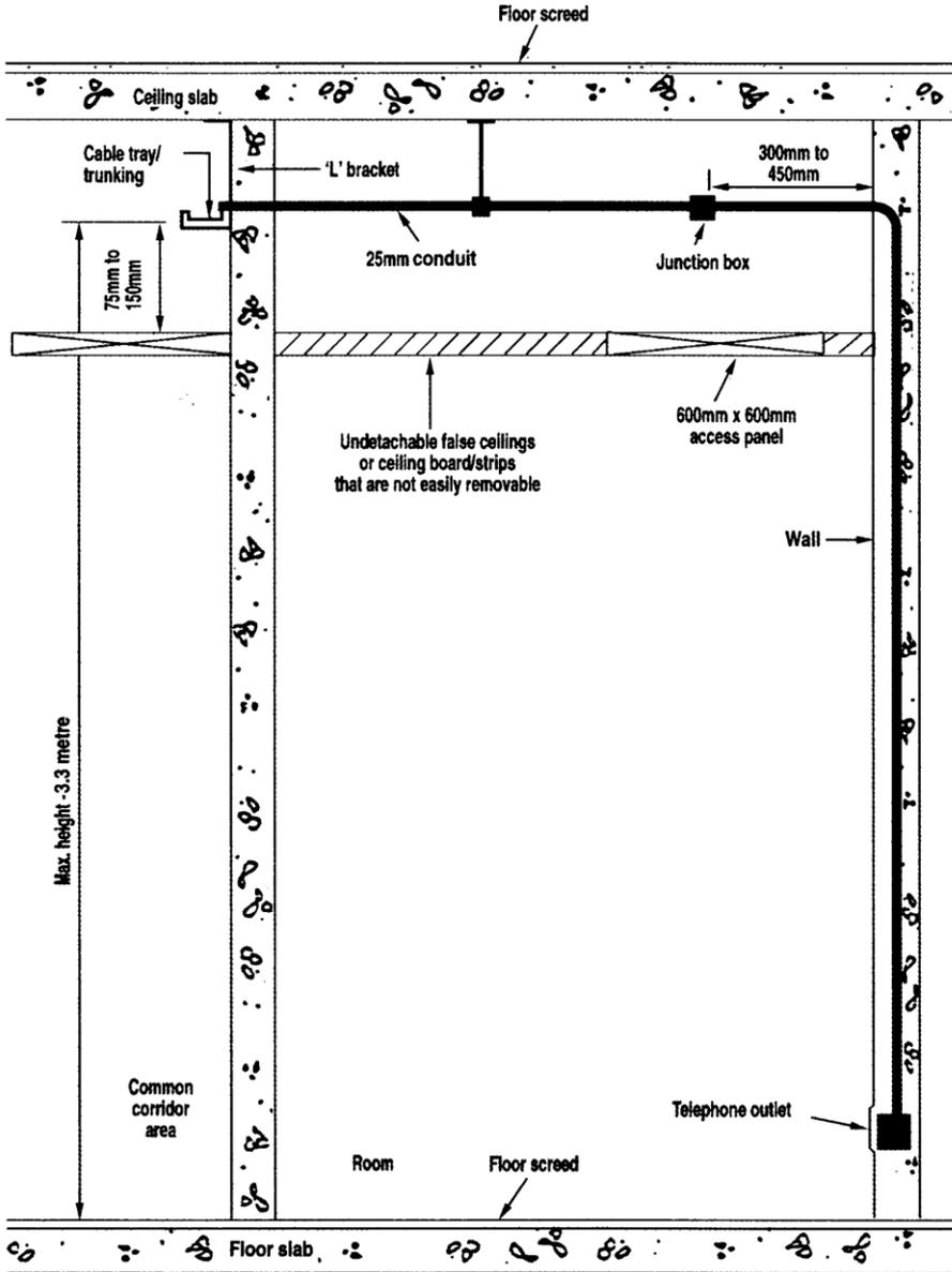
**Figure 7.18: Clearance between cable tray / trunking & obstructions**
