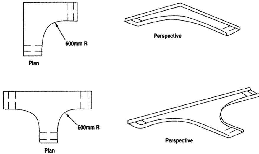
**Figure 7.27: Typical example of a trunking system**
