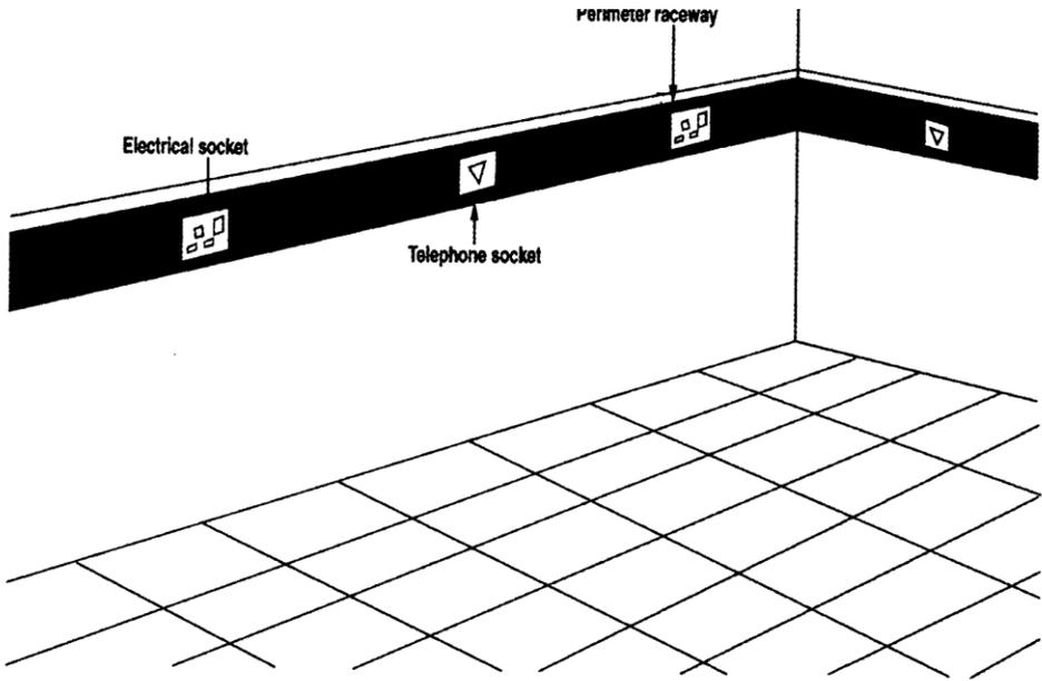
**Figure 7.20: Perimeter raceways mounted at floor level**
