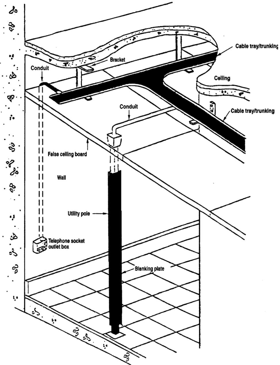
**Figure 7.17: Ceiling distribution system – Typical detail of cable tray / trunking link with conduit in non-detachable false ceiling boards / strips that are not easily removable**
