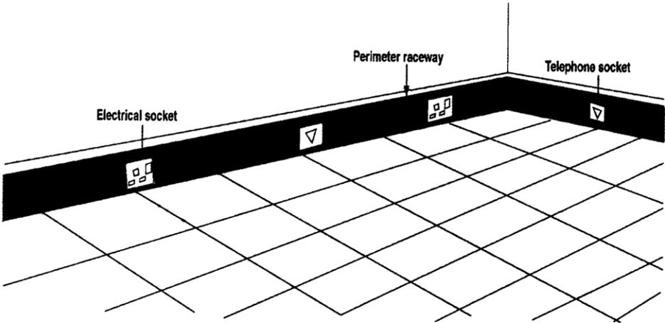
**Figure 7.21: Perimeter raceways recessed into base of wall**
