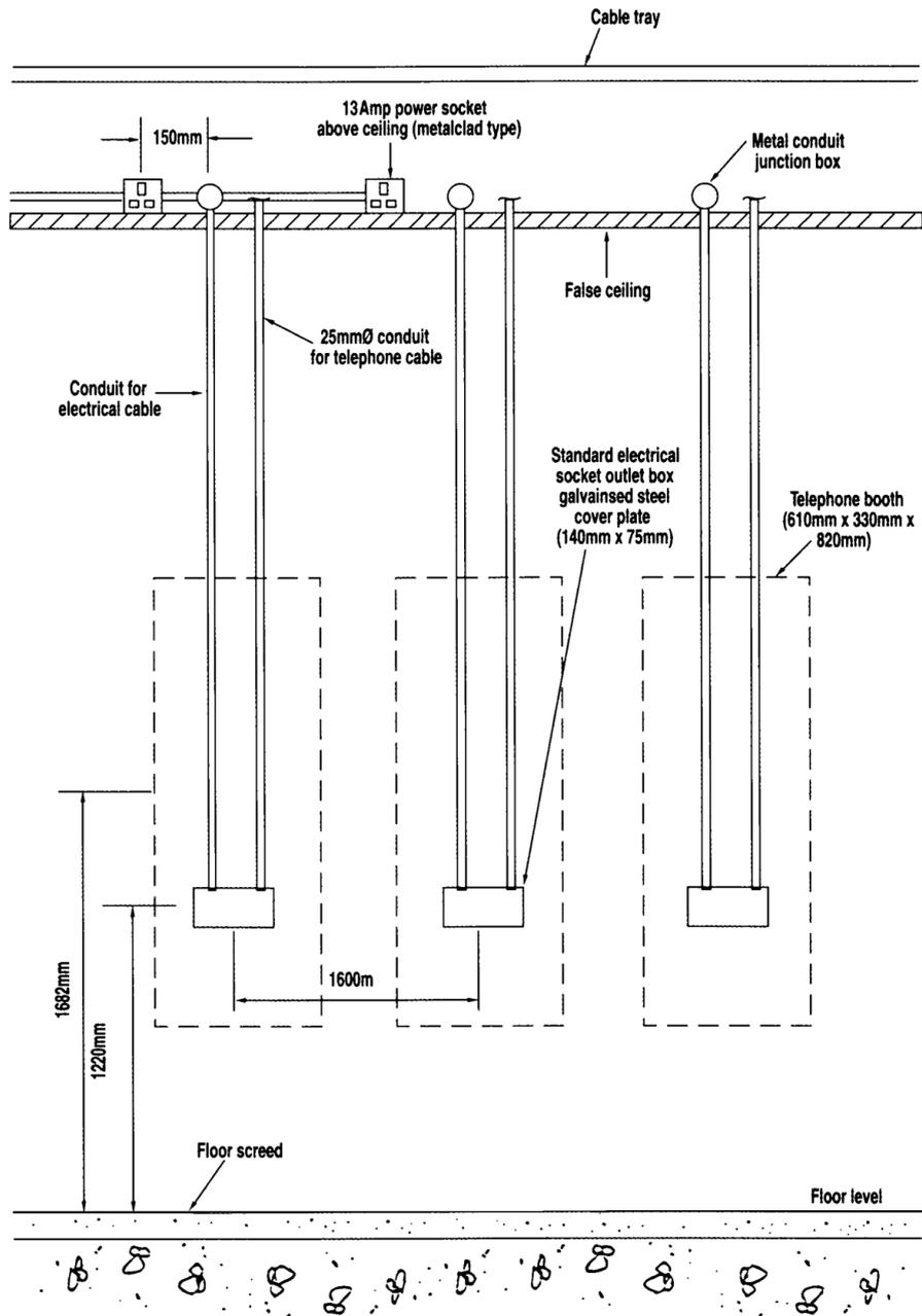
**FIGURE 5.1: TYPICAL CONDUIT FOR WALL**
