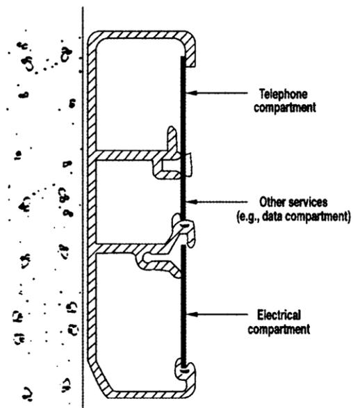
Figure 7.23: Perimeter raceways linked to under-floor duct distribution system
