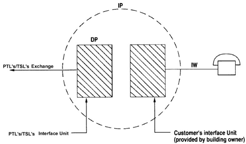
**Figure 8.3: Telephone wiring configurations for residential buildings**
