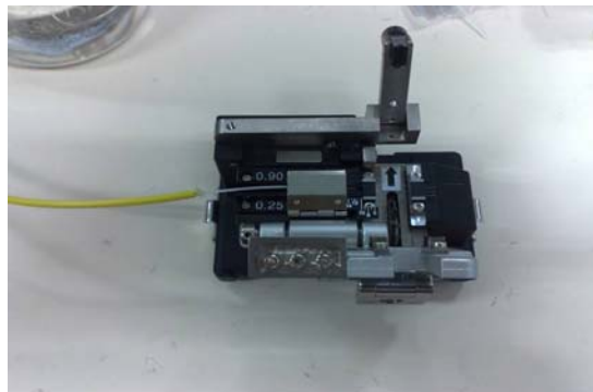
Figure 32: The Bare Fibre is Positioned and Clamped on the Fibre Cleaver before it is Cleaved
