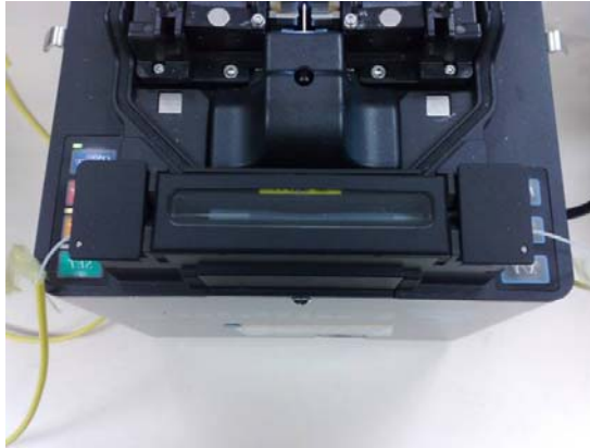
Figure 41: A Splice Protection Sleeve Heated up in the Heater (Courtesy of Fujikura Ltd)
