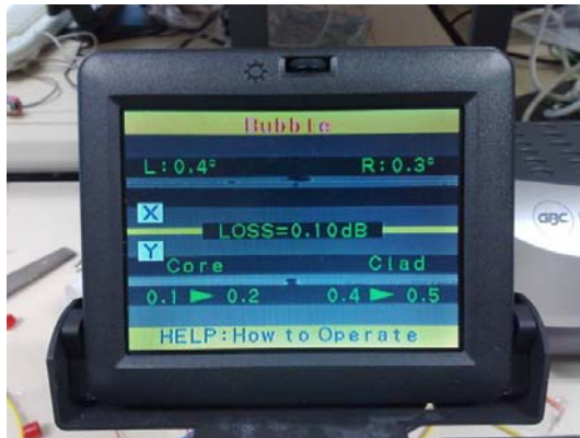
Figure 38: The Fusion Splicer Estimates the Splice Loss (Courtesy of Fujikura Ltd)
