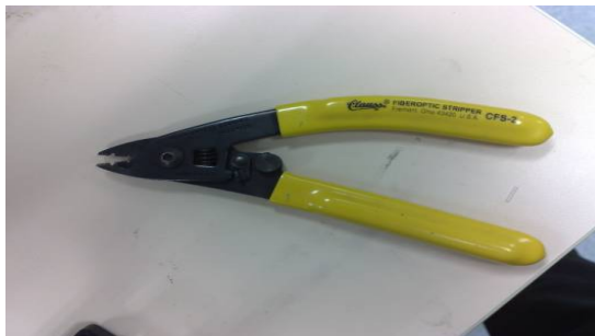
Figure 26: Photograph of a Fibre Stripping Tool for Removing the Jacket and Primary Buffer Coatings
