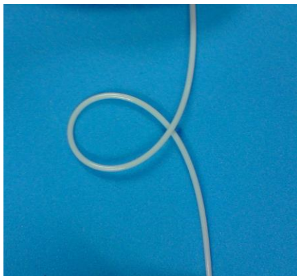
Figure 14: Example of Macrobending
