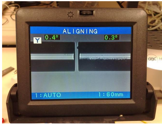
Figure 38: Photograph Showing the Process of Core Alignment (The readings of 0.4° and 0.3° are the flatness of the fibre endfaces) (Courtesy of Fujikura Ltd)
