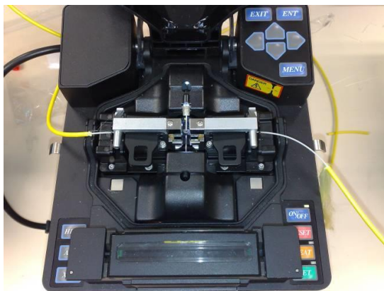
Figure 37: Photograph Showing When Both Fibres are Loaded and the Sheath Clamp is Closed (Courtesy of Fujikura Ltd)
