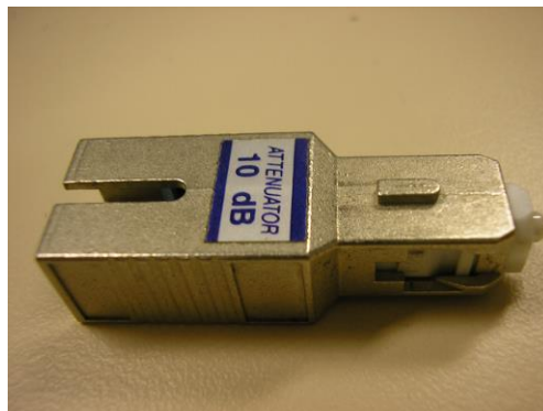
Figure 17: An Optical Attenuator in the Form of an Optical Fibre SC-SC Adapter
