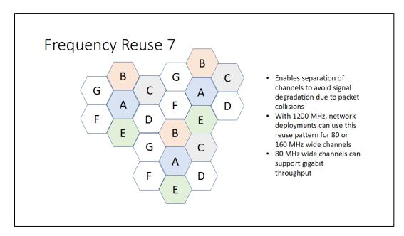
The frequency reuse 7 methodology minimizes packet collisions that degrade throughput by keeping "like" channels separated. With the full 1200 MHz available, government and enterprise deployments have access to up to fourteen 80 MHz wide channels and up to seven 160 MHz wide
