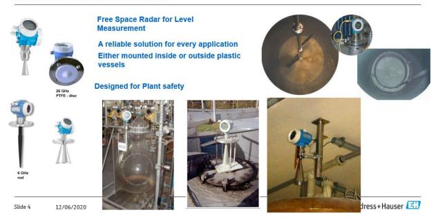
In most instances, the electronic sensors are mounted on top of enclosed vessels directed at a downward direction where interference towards external LAN signals are either negligible or non-existence.
