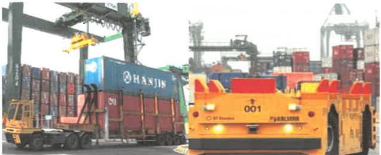
Fig 2.3.1: Conventional Prime Mover (L) versus driverless AGV (R).
