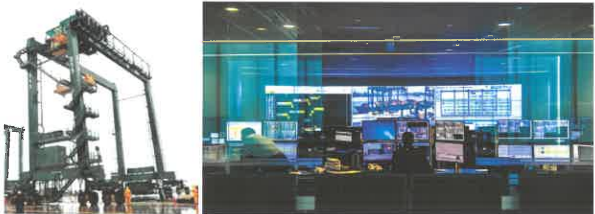
Fig 2.3.2: Conventional Yard Crane (1 operator on site per machine) (L) versus Automated Yard Cranes (remotely operated with up to 1:10 man to machine ratio) (R).
